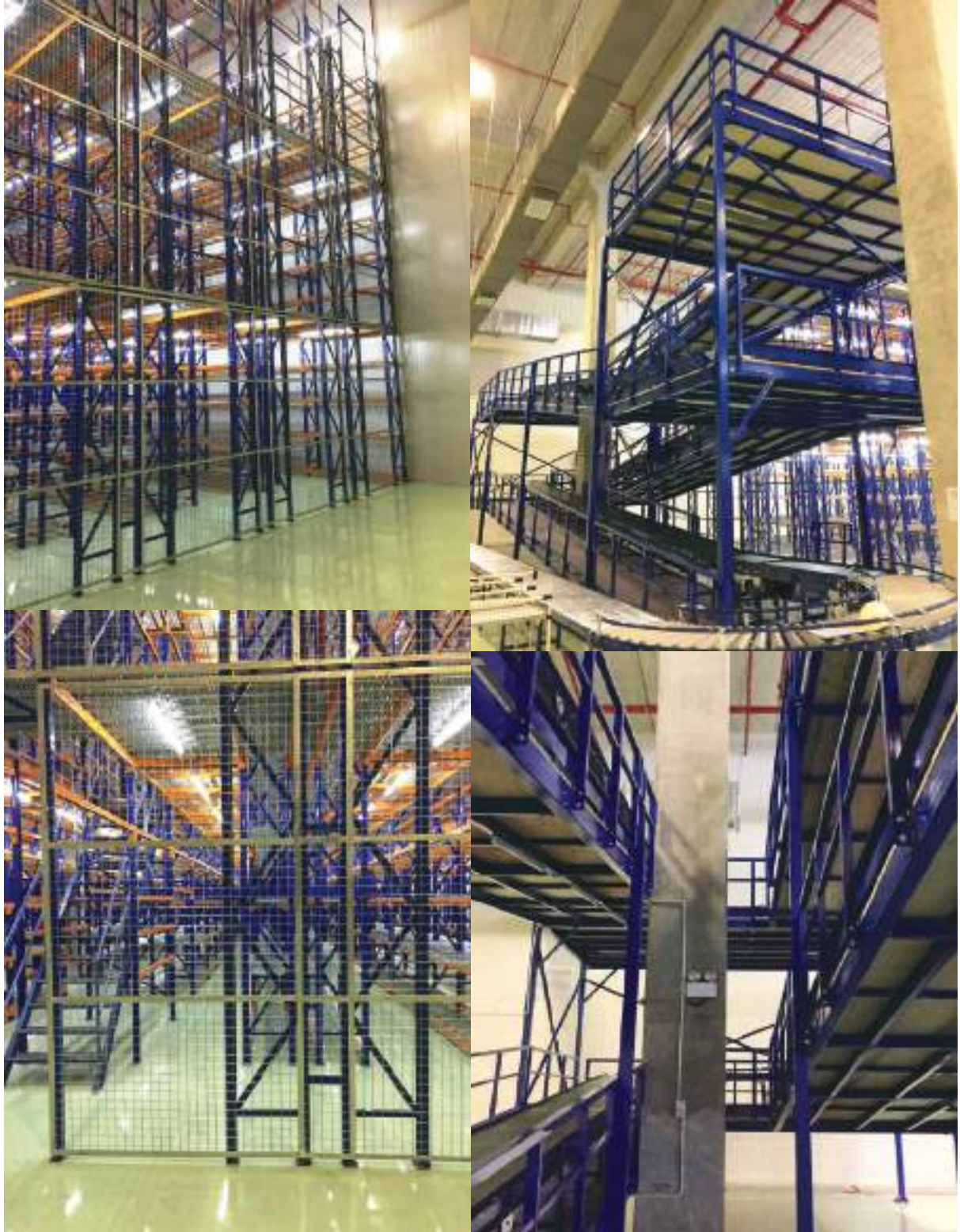
HDGI Netting & Platform
